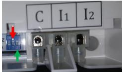
**NOTE:** For the Dip Switch setting to take effect the power and battery will need to be disconnected and reconnected.
